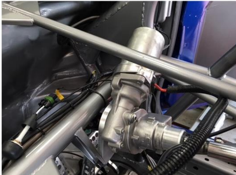
Typical MGU Installation using rear mounts and custom bracket
